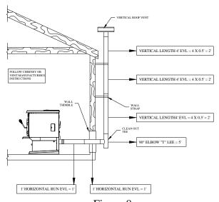
Figure 8 Venting trough wall
